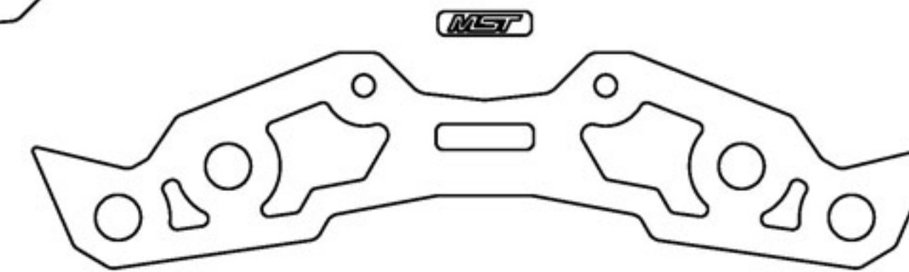
Carbon bumper support L 2.5 碳纖維泡綿壓板 2.5 L 210391
