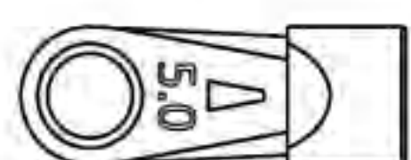
Damper adjuster 5.0 ×4 避震器拉桿
