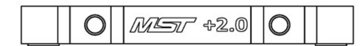
Alum. suspension mount (+2.0) ×1 鋁合金擺臂座 (820038)
